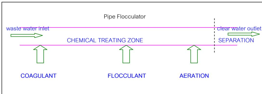
The mixing and reaction between chemicals and contaminant particles take place in a pipe, by means of controlled, calculated turbulence.
