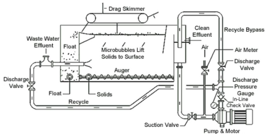
**DAF sizing** takes into consideration many criteria for sizing: Flow rate Water temperature Waste characteristics Chemical pre-treatment Solids loading (LBS/HR/Ft<sup>2</sup>) Hydraulic loading (GPM/FT<sup>2</sup>) Air to solids ratio (LBS of air/LBS of Solids)
